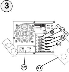
See Hardwire Electrical Connections, pg. 9. 3.1 is the cover plate, 3.2 is the five-position terminal strip, 3.3 is the output neutral (white), 3.4 is the output hot (black), 3.5 is the ground (green), 3.6 is the input neutral (blue) and 3.7 is the input hot (brown).
